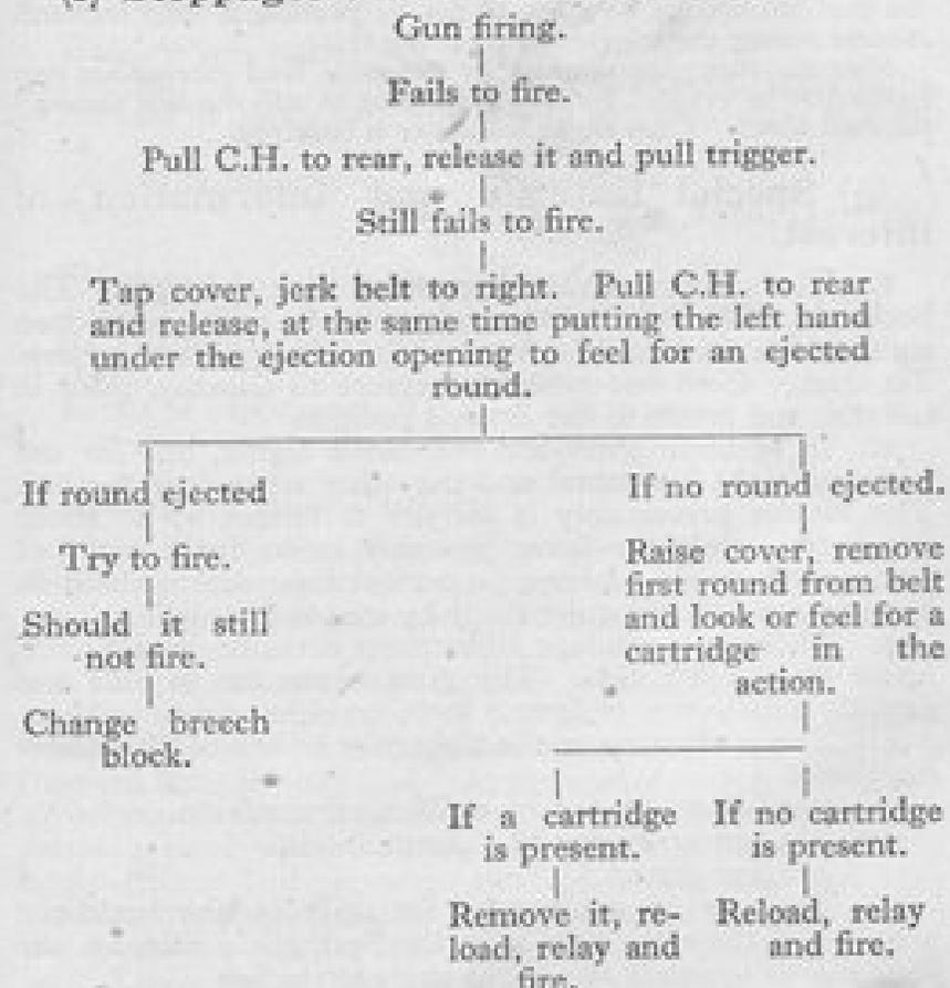
If the above does not produce any result look for breakages in, or damage to, the feed mechanism. Failing that it may be a separated case which must be cleared by means of the clearing plug.
