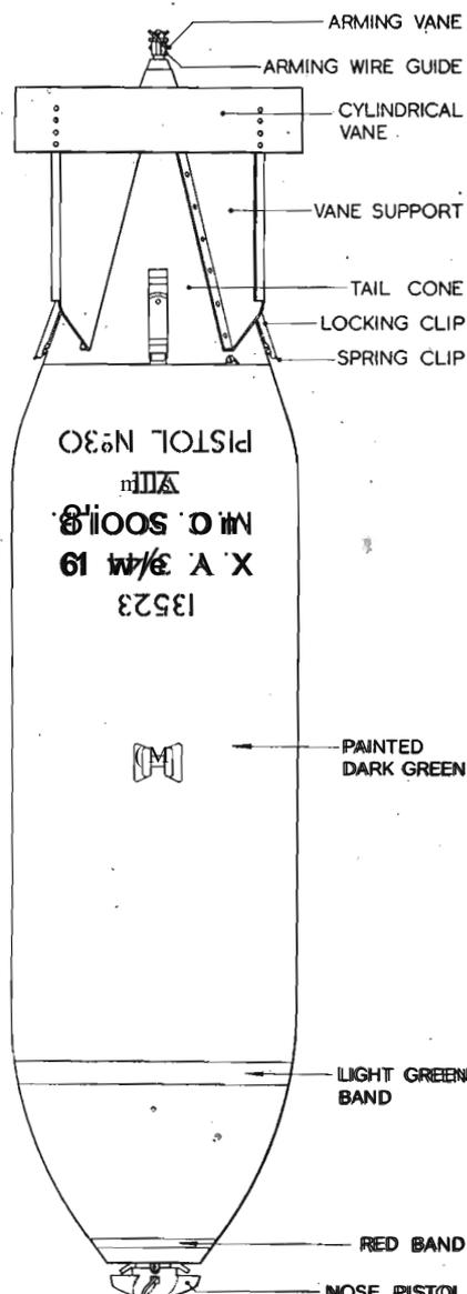
Fig. 2.—Mk. VIII bomb fitted with nose pistol and No. 28 Mk. II tail unit
