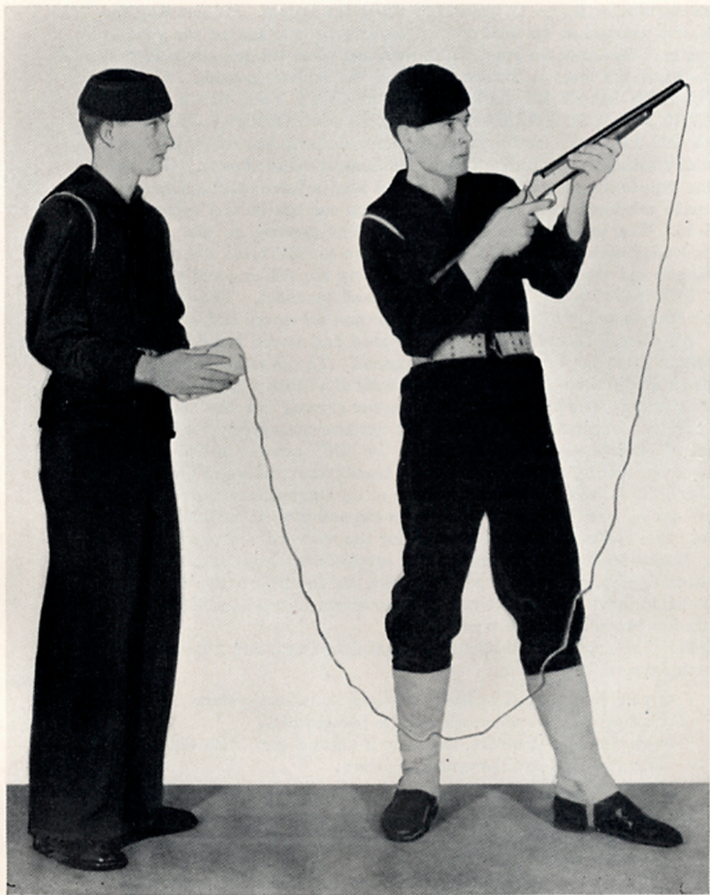
PLATE 28.—Method of use of 45-caliber line-throwing apparatus.
