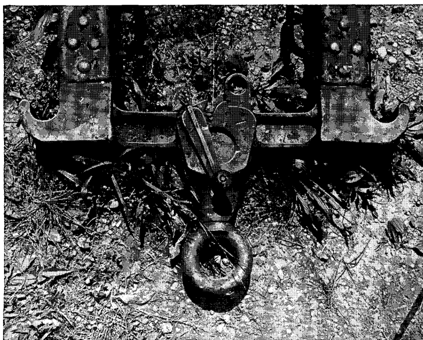
Figure 44. Trail ends in traveling position, with lock closed.
