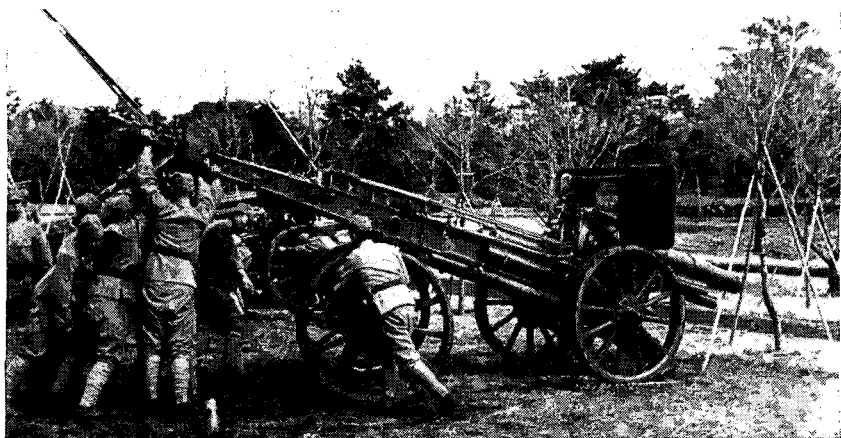
Figure 54. Assembly of Model 4 (1915) 150-mm howitzer: removing wheels of the rear trail and tube carrying section. Note position of removable rails, which carry tube from traveling position on rear trail section, to battery on sleigh of carriage.
