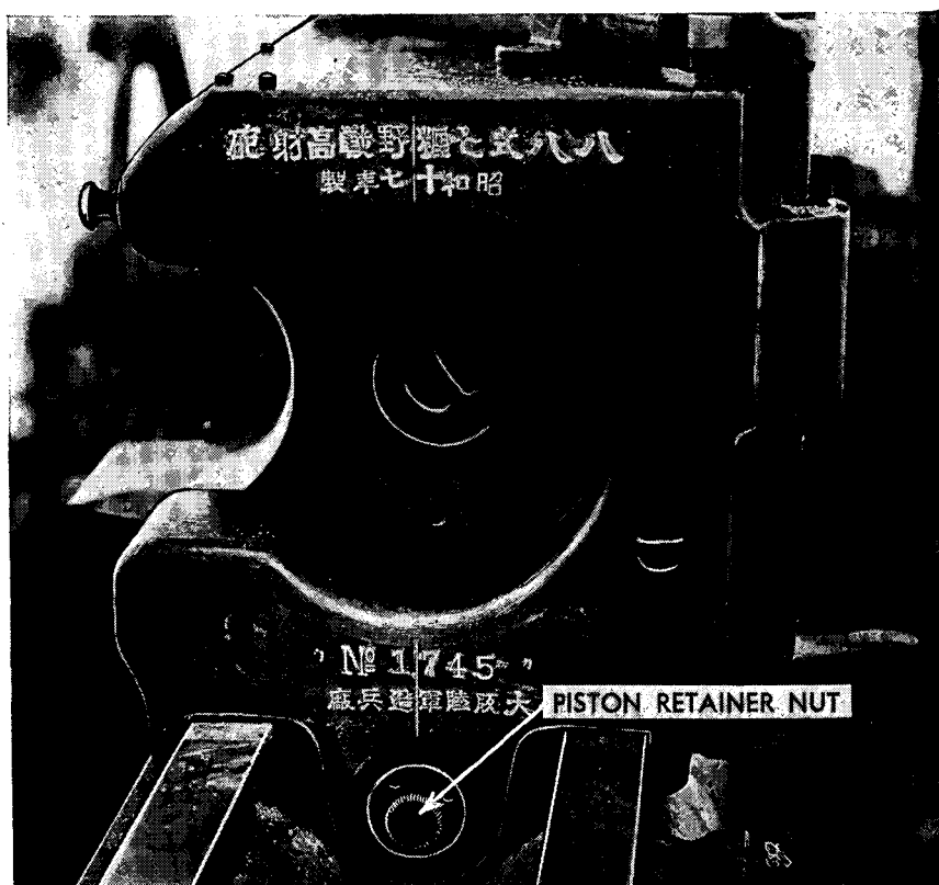
Figure 109. Breech of Model 88 75-mm AA gun, showing piston retainer nut.
