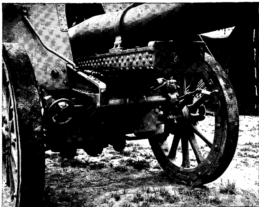
Figure 61. Model 96 (1936) 150-mm howitzer: (1) left side, showing sight mount and traversing hand-wheel; (2) front detail, showing recoil mechanism and brake lever.
