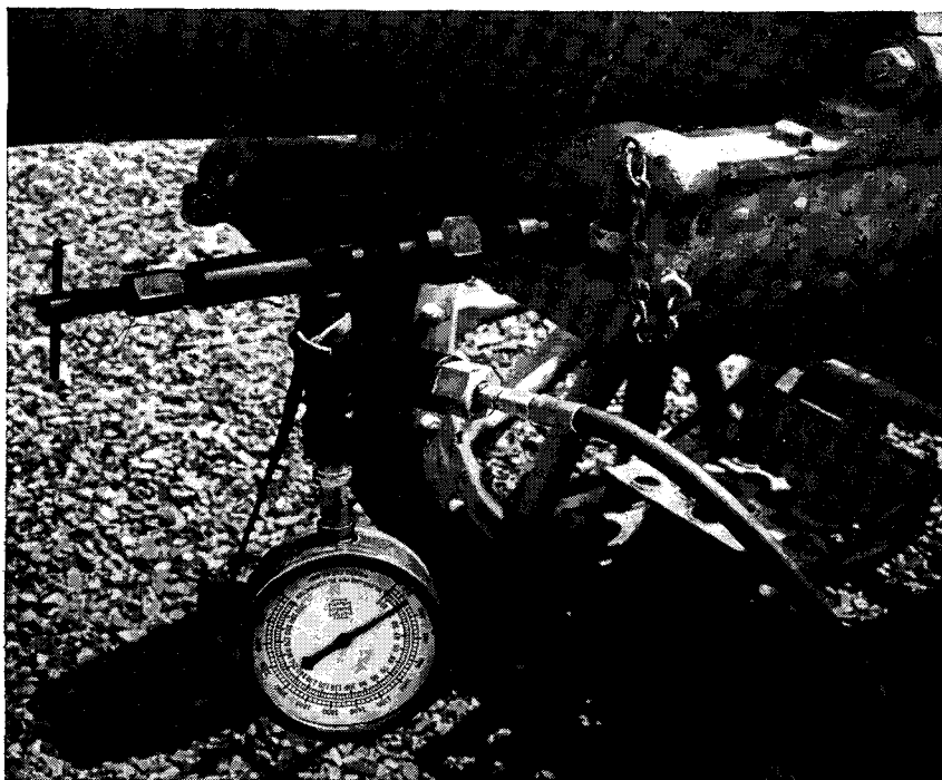
Figure 111. Front end of cradle with adapter (see fig. 102) air-filling tube (C61285), air-filling tube, flexible (C419), gauge (B147), in position for reestablishing gas pressure in counterrecoil system.
